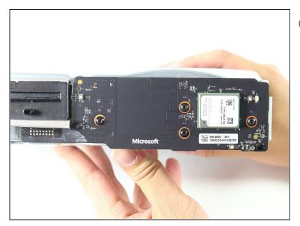
(i) The IR blaster can be identified on one of the sides of the interior case. It will be next to the disc drive and near the fan.
