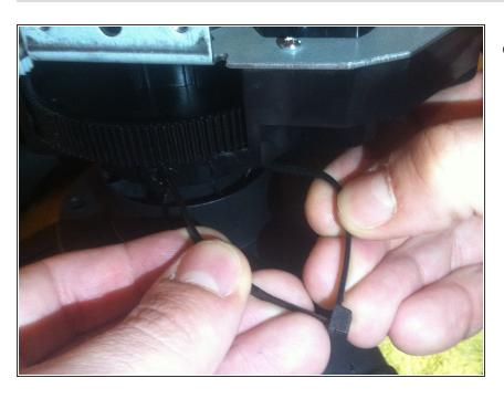
So its time to pass the zip ties around the broken plastic and remove the *loose* or *play* feeling.
