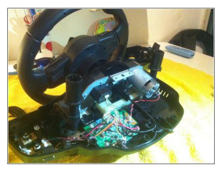
Remove Phillips Head Screws and open the cover. Before you touch anything be sure to touch a grounded object. It will be just fine to remove the static electricity, you may have.
