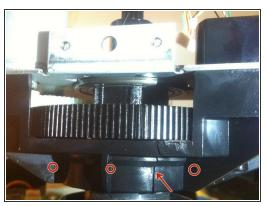
So here is the crack and we are ready to take the wheel apart. The crack is the reason for your loose or play feeling of your wheel. The red circles indicate the spots, where you should open holes with your solder iron! Through these holes the zip ties are going to pass around and make the plastic strong again!
