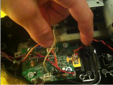
Unplug the cables from the board and be sure to remember where they fit before disassemble them!
