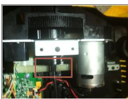
• Remove the Phillips Head Screws that hold the base of the steering wheel.Before you remove the wheel please be cautious to remember where the gears attach each other. So it would be very nice if you mark the spot where they are in touch. When you assemble the wheel attach the gears in the same place as they were from factory.
