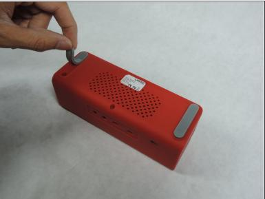
Peel off the two gray tabs to expose the four inner Philips #1 screws.
