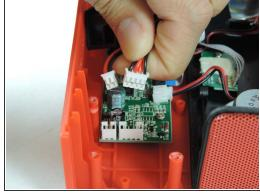
Disconnect the battery connectors attached to the circuit board by unplugging them.
