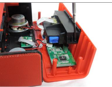
Remove the two Phillips #1 screws found on each side of the battery compartment.
