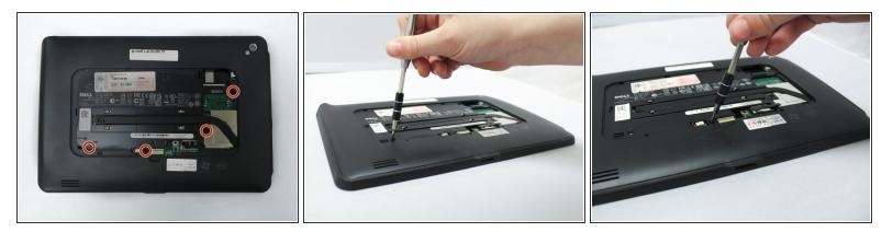
Using a Phillips #0 screwdriver, remove the four 6mm screws attaching the inside panel to the device.
