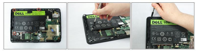
• Remove the three 6mm Phillips #0 screws attaching the battery.
