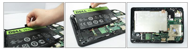
• Pull up on the black tab located at the top of the battery to remove the battery from the device.
