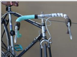
Press down on electrical tape to secure it.
