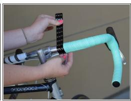
• Use the electrical tape provided to tightly secure the end of the wrap.
