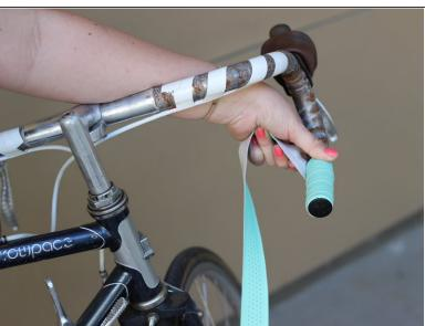
After a few wraps, tuck the extra bar tape into the end of the handlebar and firmly push in the bar end plug.
