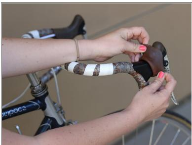
Flip the hood of the brake lever upwards.
