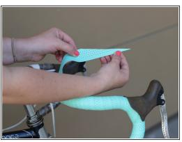
• Cut the bar tape diagonally at an approximately 60 degree angle.
