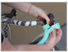
Take the extra piece of bar tape provided and cut it to fit the back of the brake lever.
