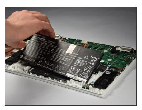
Lift the battery out by pulling upward.
