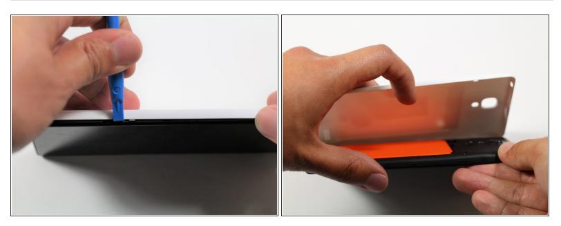
• Run the plastic opening tool along the seam on the side of the phone to remove the rear casing.
