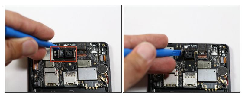
Disconnect the rear-facing camera from the motherboard by pulling out the press-fit connector to its left.
