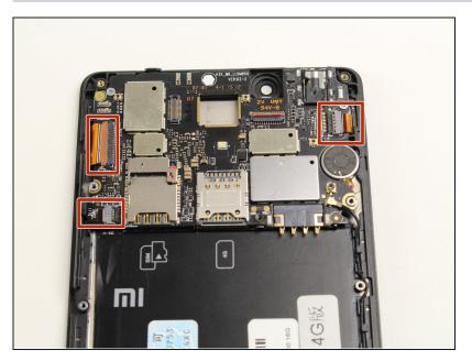
• Locate the three ZIF connectors on the motherboard.
