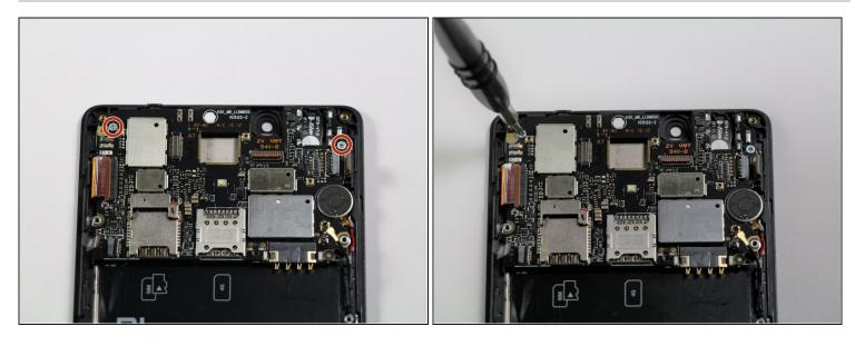
• Remove the two 2.9mm Philips #00 screws.
