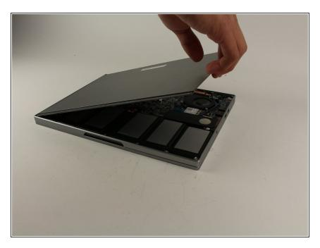
Carefully lift the back panel off of the device.
