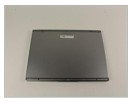
Peel off the black rubber strips from top and bottom of the back panel.
