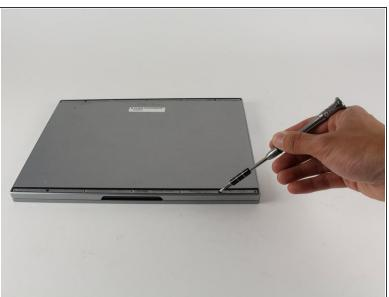
Remove the fifteen 3 mm Phillips #00 screws from the back panel.
