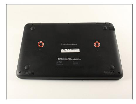
Using <u>tweezers</u>, remove the circular stickers that are covering the two screws near the middle of the back cover. Stick them to the laptop next to the screws.
