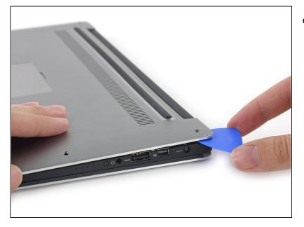
• Use opening picks or a plastic pry tool to pry open the case clips, beginning from the back edge.
