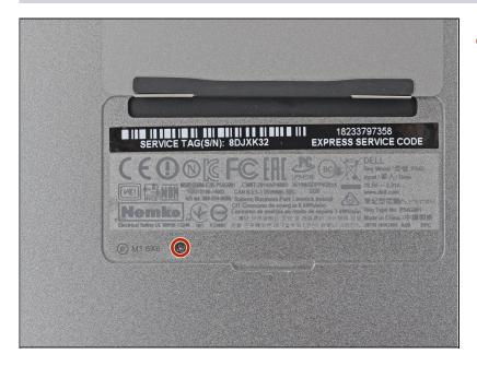
• Remove the single Phillips screw hidden beneath the flap.
