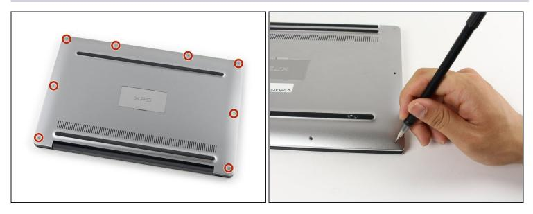
Remove the eight 4 mm T5 Torx screws from the bottom cover.
