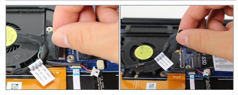
• Remove the black standard flat connector by lifting the tab up with your hand.
