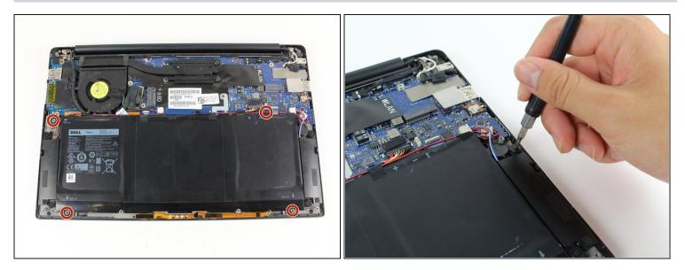
• Remove the four 3 mm Phillips #0 screws located on each corner of the battery.
