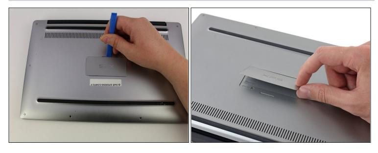
• Use a plastic opening tool to pry open the 'XPS' flap in the middle.
