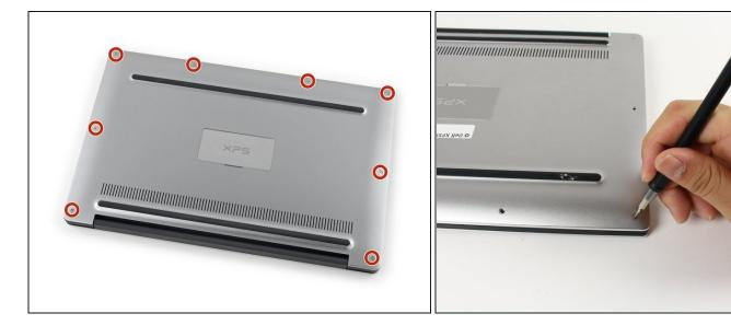
• Remove the eight 4 mm T5 Torx screws from the bottom cover.
