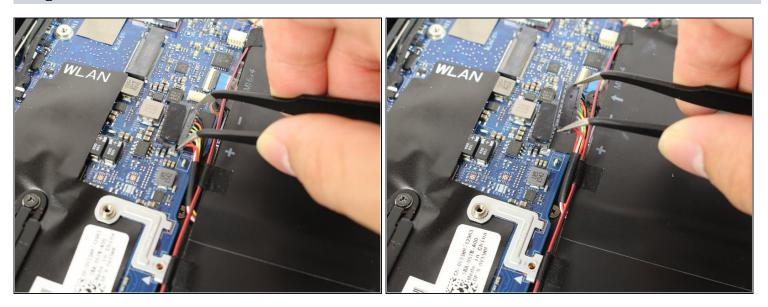
• Pull the battery cable connector towards the battery to disconnect it from its socket.
