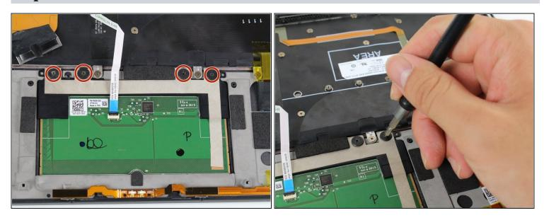
• Remove the four 3 mm Phillips #1 screws from the trackpad.
