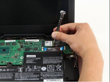
• Use a Philips #1 screwdriver to remove the 3.6 mm screw from the back panel.
