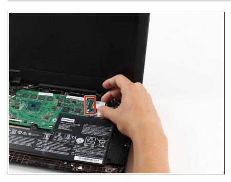
Gently slide the wireless card to the right to remove it from the standard socket on the motherboard.
