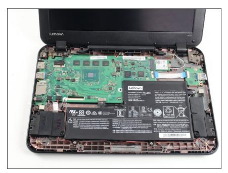
Lift the keyboard up and off the back panel, exposing the motherboard and battery.
