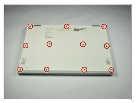
Using a Phillips screwdriver, remove all eleven 7.0 mm screws from the bottom of the Chromebook.
