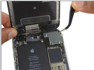
• Remove the display cable bracket.
