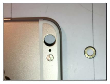
Insert new ring with tiny dots of super glue. Don't use too much glue and get it on the frame.
