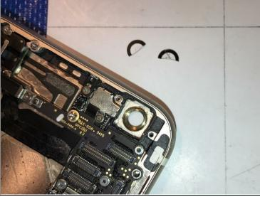
• Remove the glass by pushing out from the inside of the frame
