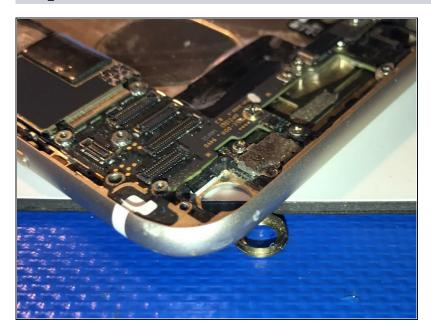
Once ring is out of the frame, there should be no bending at all on the frame.
