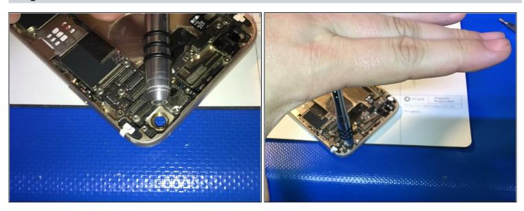
• Use a driver without a bit to fit on the ring from the inside. *It shouldn't rest on the frame around the ring at all.* Gently tap down on the ring until it pops out while firmly holding the frame down.
