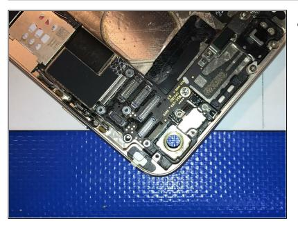
Butt the lens rim up against a raised surface with the rest of the phone on the surface and the ring over air.
