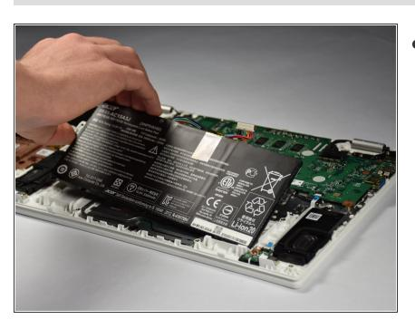
Lift the battery out by pulling upward.
