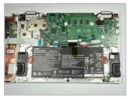
Remove the two 4.5 mm Phillips screws located at the sides of the battery.
