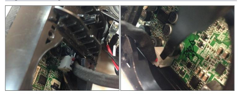
• Using <u>tweezers</u>, carefully remove both side speakers from the motherboard as shown in the pictures.
