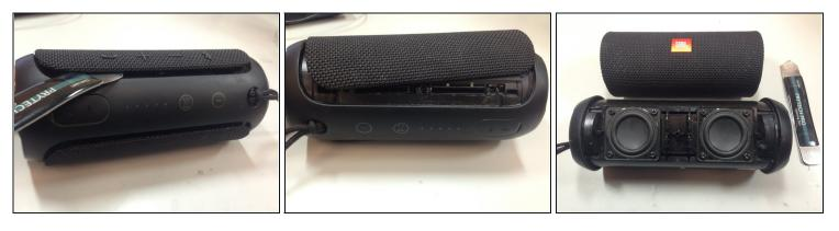
• Continue to pry open the grill all the way around until it can be removed from the unit itself as seen in the pictures.
