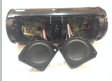
• Using a pry tool, remove speakers from housing as seen in the picture.
