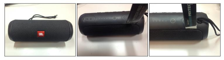
Using a pry opening tool, pry into the speaker grill covering as seen in the photos.
