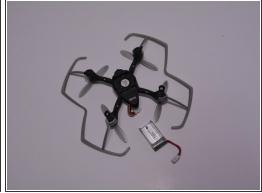
Pinch the side of the battery that is already exposed and pull until the battery is fully removed from the drone.
