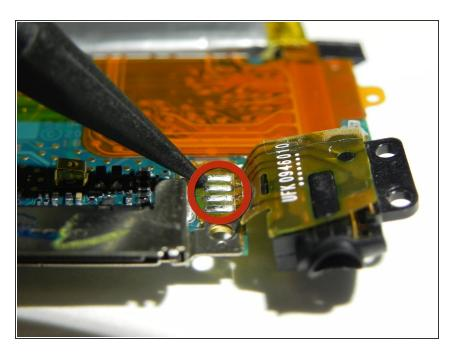
Solder the new headphone jack onto the logic board, making sure to solder all five points.
