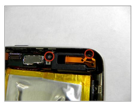
Remove the remaining two Phillips screws in the top right corner and the top center.
