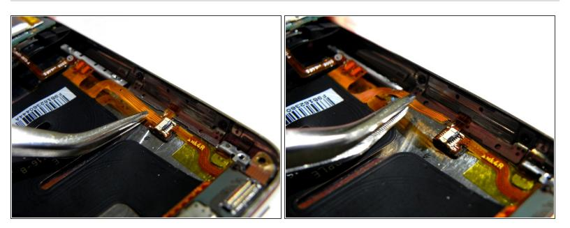
Once the switch is flipped, remove the ribbon from its socket by gently pulling the ribbon straight out with tweezers.
