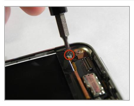
Remove the Phillips screw in the top left corner attaching the metal tray to the rear panel.
