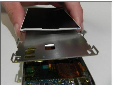
Lift the metal tray slightly (the battery is attached to the underside) and remove the display from the iPod.
