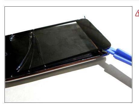
Make sure not to slide the tool along the edge once you've managed to wedge it between the screen and panel. Repeat the process of prying the tool into a point along one of the edges and remove the tool to insert it at another point.
