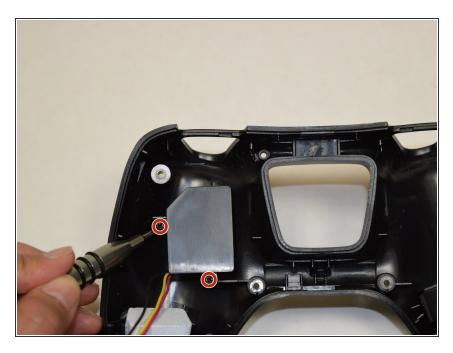
Use a screwdriver to remove the two 0.7 mm screws from the battery cover.
