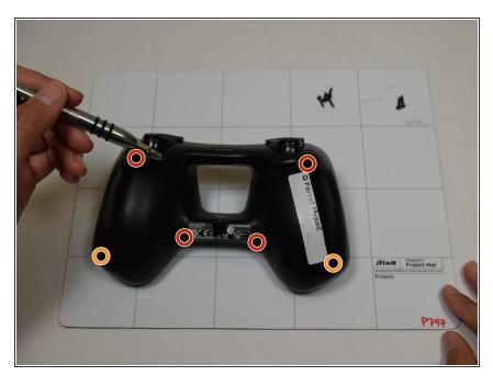
Use a T6 screwdriver to remove the six screws from the back of the controller: four 0.9 mm screws and two 0.1 mm screws.
