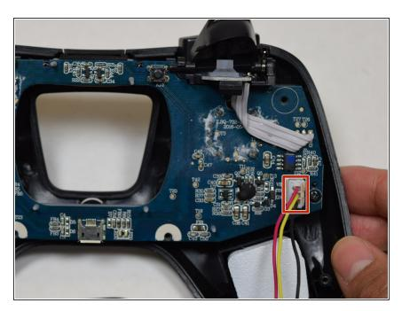
Gently attach the wire connection from the new battery to the motherboard. Avoid touching the motherboard directly.
