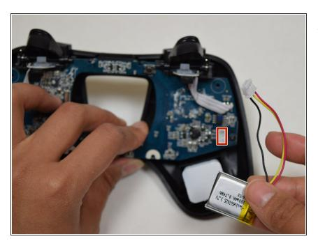
Use fingers to gently detach the battery wires from the motherboard.
