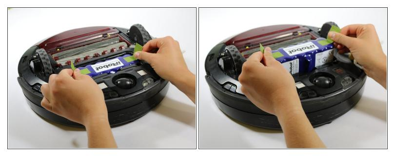
• Remove the battery using the green tabs on either side of the battery.
