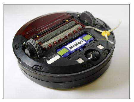
• Remove the battery cover and place it off to the side.
