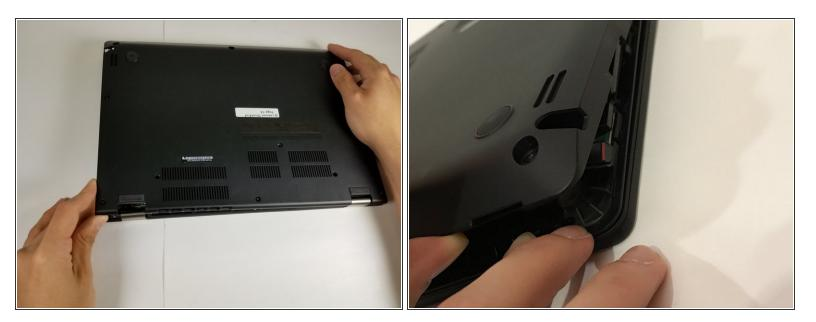
After removing all of the screws, gently lift up on all covers to remove the back plate and reveal the interior of the device.
