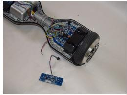
• Carefully remove the gyroscope component from the SwagTron.
