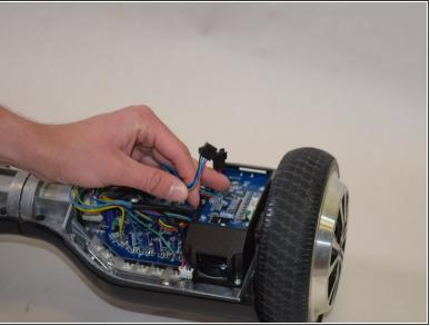
Disconnect the gyroscope by disconnecting the wires attached to it. These wires are black, green, blue and red.
