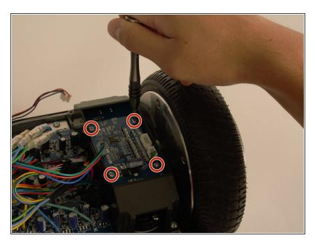
Using your Phillips #2 screwdriver, remove the four 8mm screws marked in red from the gyroscope.
