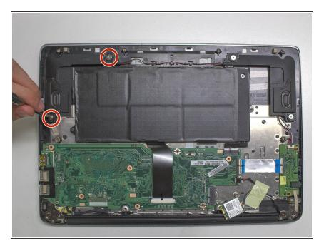
Remove the two 4mm Phillips #0 screws securing the speaker.
