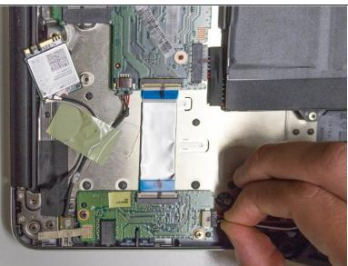
Disconnect the speaker wire from the circuit board by grabbing the plug by its plastic edges and gently pulling it straight out.
