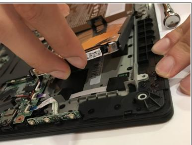
Using two fingers, carefully remove the hard drive.
