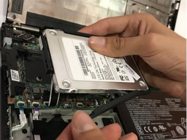
Carefully remove the plastic encasing surrounding the perimeter of the hard drive.
