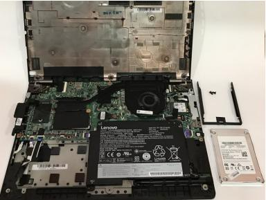
After the SATA connection is removed, gently pop off the hard drive from its socket.
