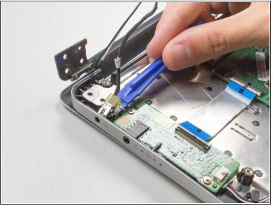
Remove the power port entirely from the computer by pulling up on the plastic portion of the port with a plastic opening tool. To reassemble your device, follow these instructions in reverse order.
