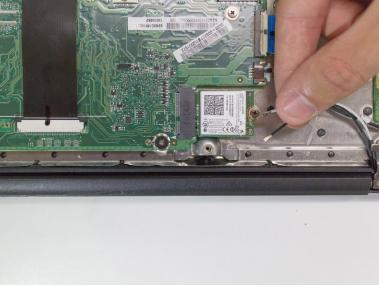
Disconnect black and white wires from the wireless adapter by gently pulling up on the metal connectors with your fingernail.
