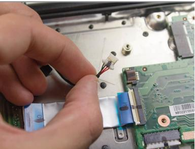
Detach the power port plug from the main circuit board by grabbing it by the sides of the plastic with the tweezers and gently pulling it out.
