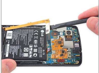
Use the flat end of a spudger to disconnect the daughterboard ribbon cable and pull it away from the battery.
