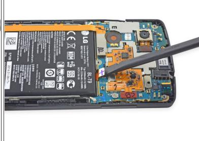
Use the flat end of a <u>nylon spudger</u> to disconnect the battery connector.
