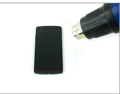
Use a heat gun or an iOpener to soften the adhesive along the edges of the screen.
