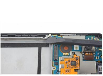
• Use the flat end of a spudger to disconnect the left antenna cable.
