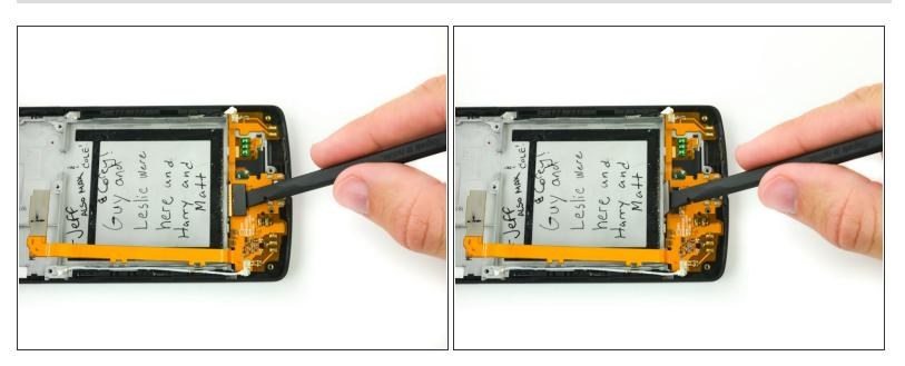
Use the flat end of a nylon spudger to pry the digitizer ZIF connector up off the daughterboard.
