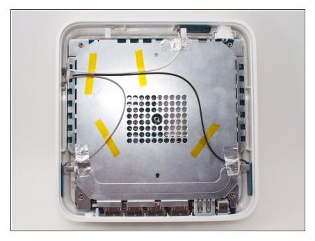
After unscrewing all five screws, remove the plastic casing. The back should now look like the picture shown.
