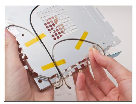
Carefully peel back the metallic silver tape covering the cable of the antenna to be removed.
