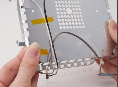
Carefully peel back the clear yellow tape covering the cable of the antenna to be removed.
