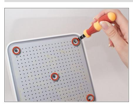
After removing the rubber covering, unscrew the five 4.9mm Phillips screws in the holes of the plastic casing.
