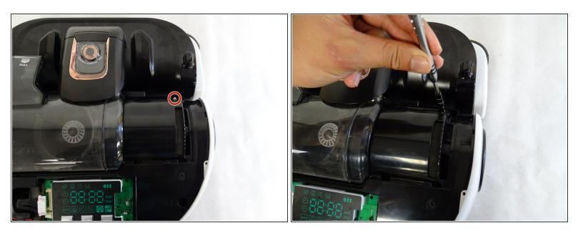
• Remove the 6mm Phillips #1 screw in the hole that was under the copper-colored vacuum cover.
