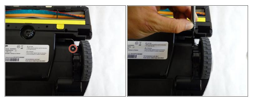
Flip the device over and remove the 6mm Phillips #1 screw in front of the left (from this perspective, right) wheel.
