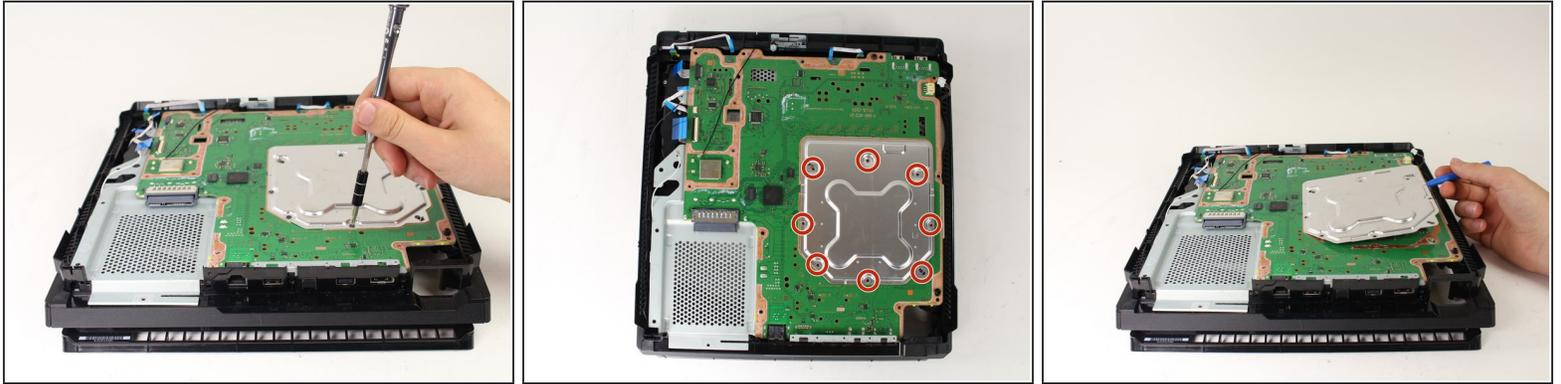
**i** If you are working on the **7200-series model**, this metal plate will have been already removed as part of the removing the larger motherboard plate. You may skip this step if this is the case.
