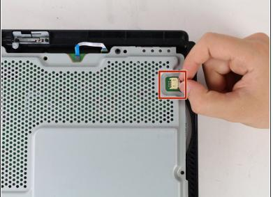
Pull the white fan connector straight out of the yellow mount on the motherboard.
