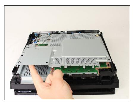
Pull up and remove the metal plate.
