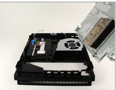
Lift the metal plate that is connected to the heat pipe straight up to remove it.
