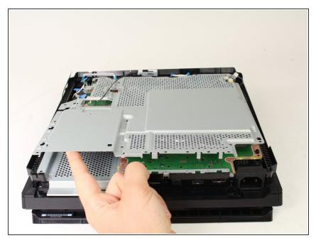
Pull up and remove the metal plate.
