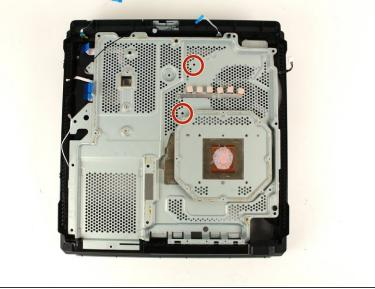
Use a Phillips #1 screwdriver to remove the two 6 mm silver screws from the metal plate.
