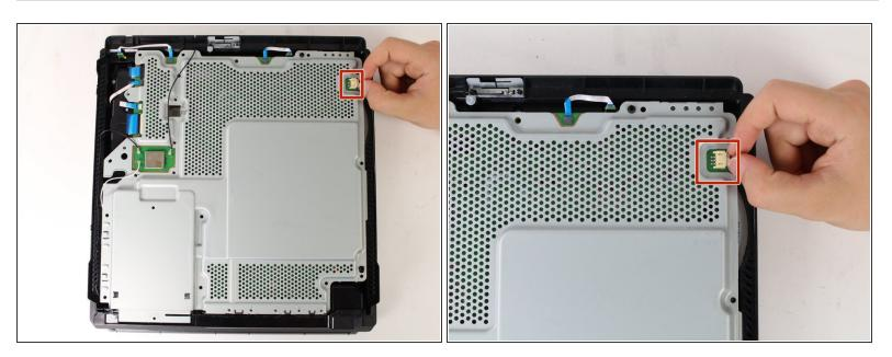
Pull the white fan connector straight out of the yellow mount on the motherboard.
