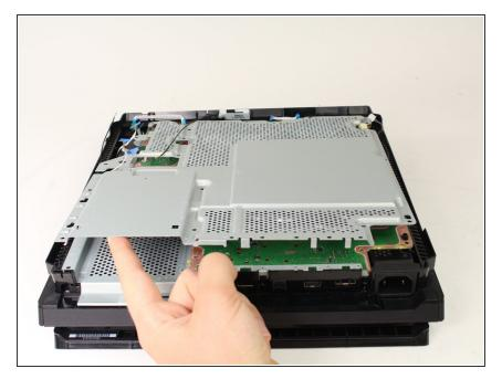
• Pull up and remove the metal plate.
