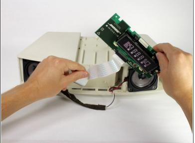
Lift the screen assembly upward and pull the white wire strip out of the device.
