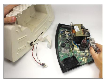
The base should now be completely detached from the device.
