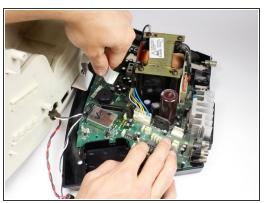
Gently pinch and pull on the white ribbon cable to disconnect it from the base.
