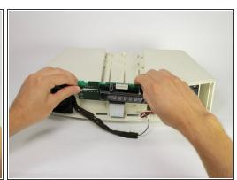
Gently pull the top of the screen assembly away from the device.
