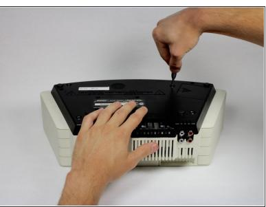
Remove the four 19mm Phillips #2 screws from the base of the device.
