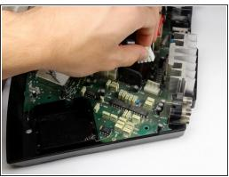
• Pinch and unplug the white connector from the device.
