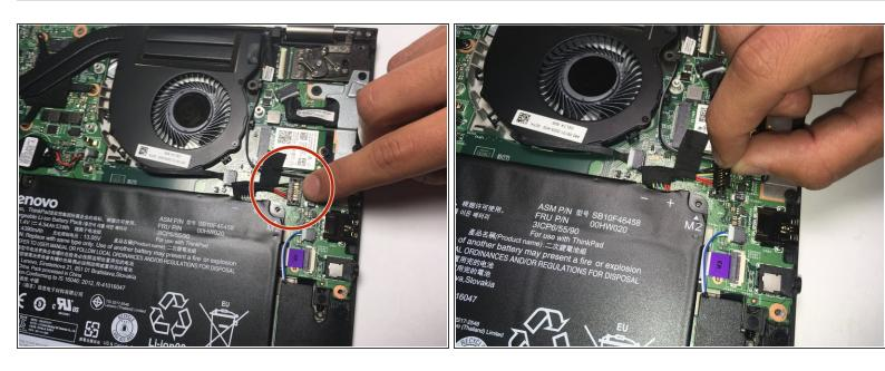
• There will also be a clip that attaches the battery to the rest of the laptop. Unclasp the clip from its holding to completely free the battery.
