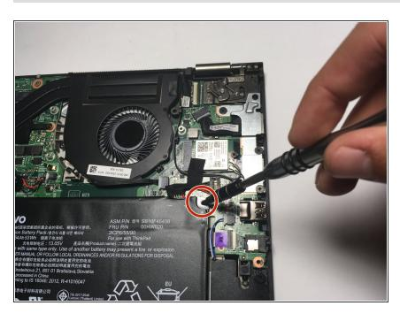
To remove the battery, use a Phillips head screwdriver to unscrew four screws. They are located at the four corners.
