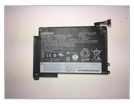
Once all wires are detached from the rest of the computer, remove the battery from the laptop and replace.
