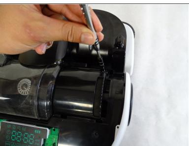
Remove the 6mm Phillips #1 screw in the hole that was under the copper-colored vacuum cover.
