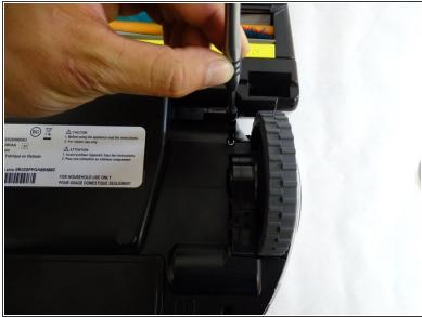
Flip the device over and remove the 6mm Phillips #1 screw in front of the left (from this perspective, right) wheel.
