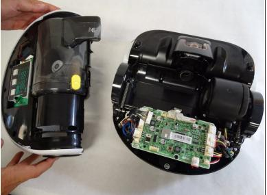
Remove the top chassis from the POWERbot by grabbing the wheel covers and lifting upwards.
