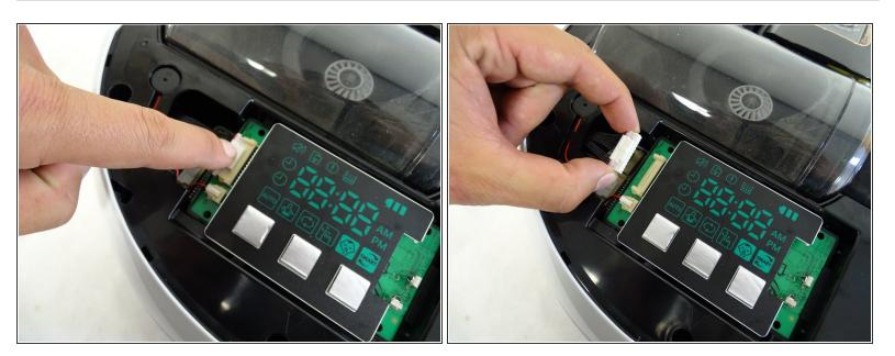
Detach the wider circuit connector by pressing down gently on the left end of the clip and pulling the connector out.
