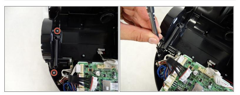
Remove the two 5mm Phillips #1 screws in the holes closest to the left wheel.
