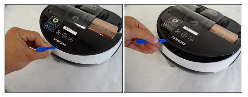
Insert the plastic opening tool under the black cover, near the Samsung logo on the back of the device, and partially pry open.
