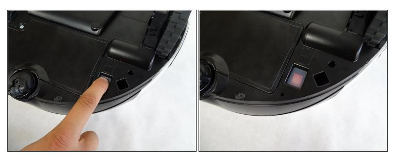
Turn off the emergency switch located at the bottom right of the POWERbot.
