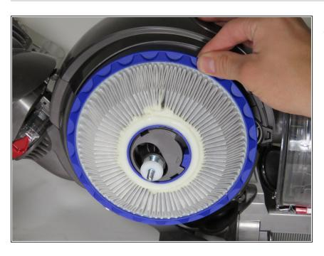
Turn 1/4 turn counterclockwise to release filter, then pull off to remove.
