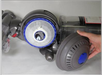
• Grip the grooves on the blue dial and unscrew counterclockwise until the side housing is free.
