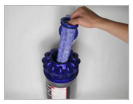
Pull the filter straight up to remove.
