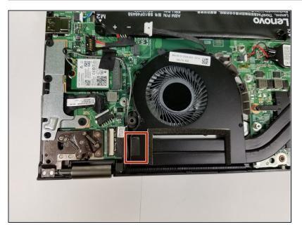
Gently peel back a piece of tape in the bottom left corner of the fan.
