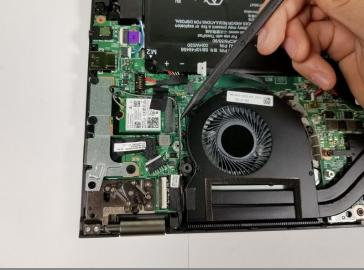
• There is a wire looped around the fan. Use the spudger to pull the wires out of the loop.
