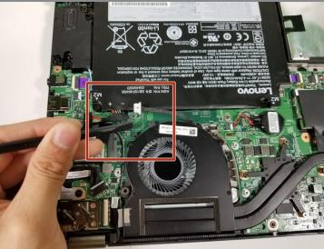
• Use the flat end of the spudger to push the connector out of its socket .
