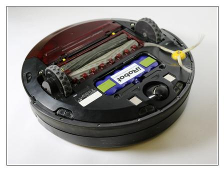
Remove the battery cover and place it off to the side.
