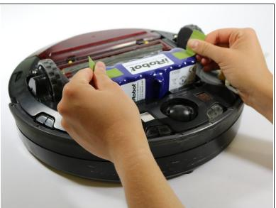
Remove the battery using the green tabs on either side of the battery.
