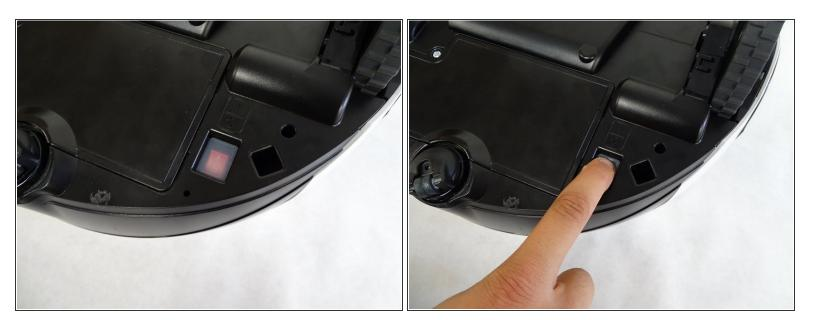
Turn off the emergency switch on the bottom of the power bot.
