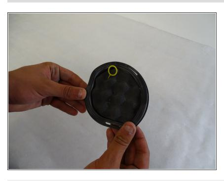
The filter is removed. You can dispose of collected dust or rinse the filter with warm water before replacing.
