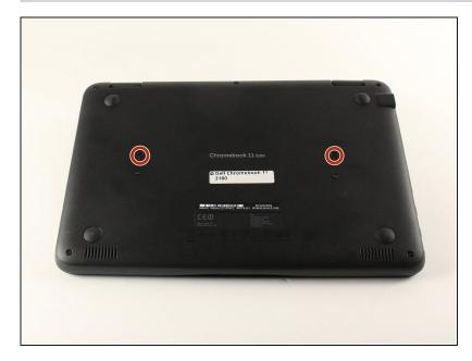
Using <u>tweezers</u>, remove the circular stickers that are covering the two screws near the middle of the back cover.
