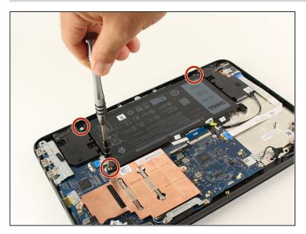
Using a Phillips #0 screwdriver, remove each of the three 3mm screws from the battery.
