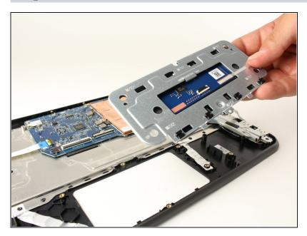
• Lift the touch pad, with it's bracket, away from the computer to remove it.
