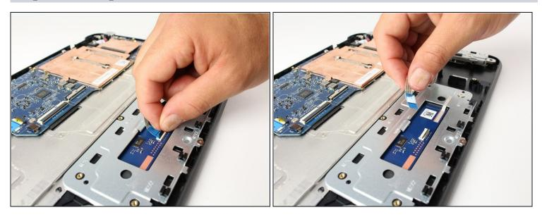
• Unplug the touch pad from itself by lifting up on the connector and pull out the ribbon cable.
