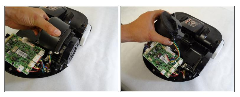
Remove the vacuum motor by grabbing the body of the motor and lifting upwards.
