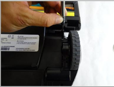
Flip the device over and remove the 6mm Phillips #1 screw in front of the left (from this perspective, right) wheel.
