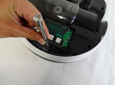
Remove the three 6mm Phillips #1 screws in the holes near the back of the device.
