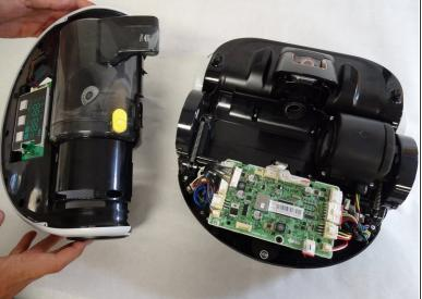
Remove the top chassis from the POWERbot by grabbing the wheel covers and lifting upwards.
