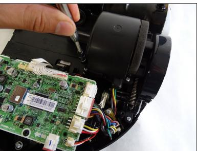
Remove the three 5mm Phillips #1 screws in the holes around the vacuum motor.
