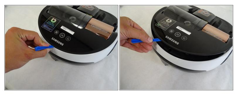
Insert the plastic opening tool under the black cover, near the Samsung logo on the back of the device, and partially pry open.
