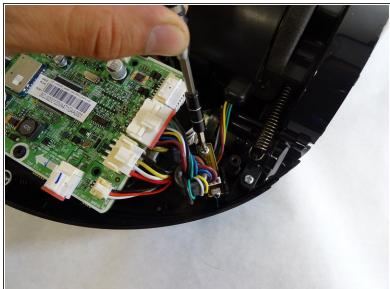
Remove the 5mm Phillips #1 screw on the peg to the right of the circuit board.
