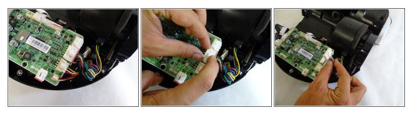
Detach the largest circuit connector on the right side by pressing down gently on the right end of the clip and pulling the connector out.
