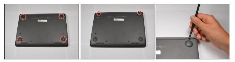
Using a sharp tool, remove the six adhesives from the bottom of your laptop to expose the screwheads underneath. Two of the pads are small and four are larger.
