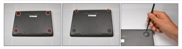
• Using a sharp tool, remove the six adhesives from the bottom of your laptop to expose the screwheads underneath. Two of the pads are small and four are larger.
