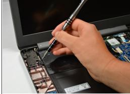
Using your Phillips #0 screwdriver, remove the five 0.2 mm screws from the battery.
