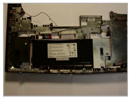
Replace the battery with a 11.1V, 7500mAh Li-ion battery, MSI part number: BTY-L77 or equivalent.
