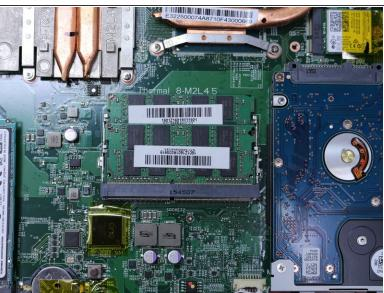
When you open the back cover, the RAM will be located as shown in the picture.
