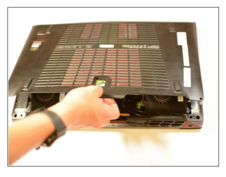
With the screws out, remove the bottom door.
