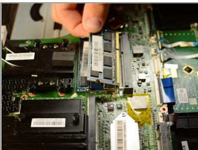
Pull back clamps holding the RAM to remove it from the socket.
