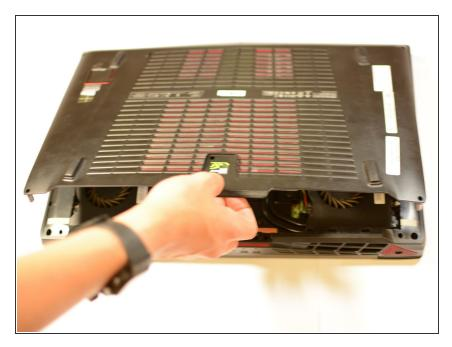
• Lift the back cover off by lifting by the tab on the bottom of the cover as indicated.
