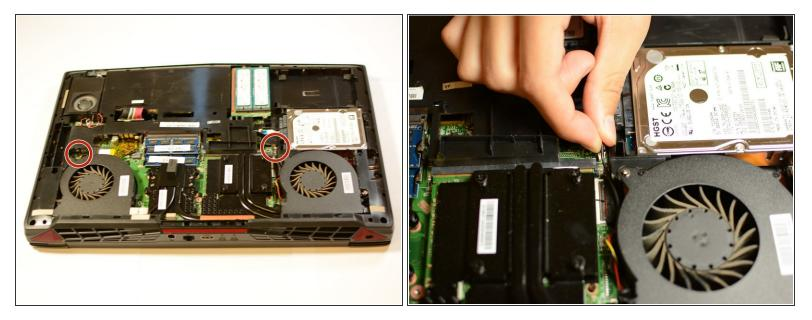
Detach the two indicated wires by pulling upward on them.
