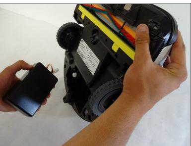
Remove the battery by holding the battery in place and partially righting the POWERbot so the battery falls out.
