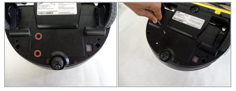
Unscrew the two 6mm Phillips #1 screws and remove the lid, exposing the battery.
