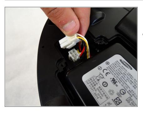
Push the tab inwards to the white box and pull the wires up. This will release the wires from the white box, allowing you to remove the battery.
